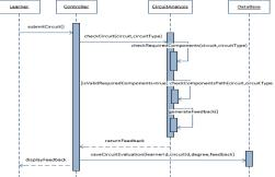
Fig. 6. UML sequence diagram for circuit analysis
